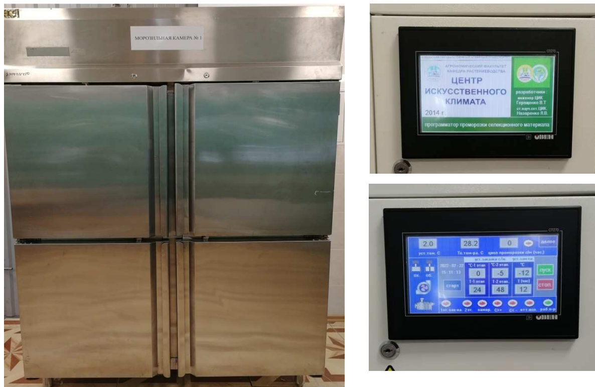
Figure 1 – EKSI freezer and programmer for a flexible freezing temperature control system
